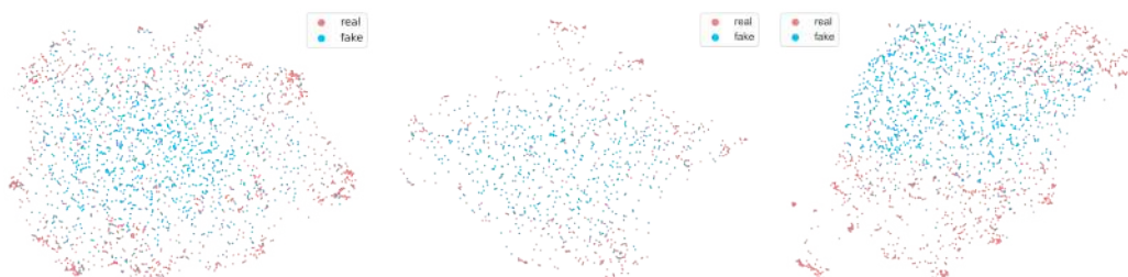
Figure 6.6 UMAP projections of “real” and generated pose samples. The plots visualize ground-truth samples alongside synthetic poses produced by SPoser (left), RVPoser [7] (middle), and VPoser [4] (right). SPoser uniquely maps human poses onto a hyperspherical manifold, enabling the use of advanced spherical interpolation schemes while achieving broader and more uniform coverage of the ground-truth pose distribution.
