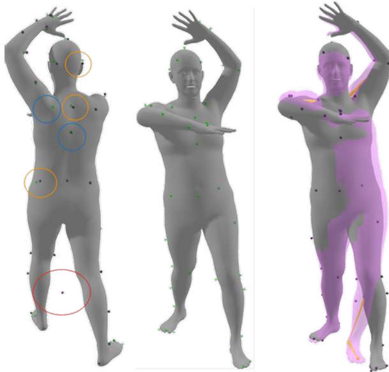
Figure 1.5 Different forms of noise are generated by the sensors (on the left side of the image) or by the AI model (in the middle). Low-cost sensors introduce measurement noise and ghosting artifacts , whereas sparse camera views cause information loss . When AI models treat observations as fully certain , this mismatch propagates uncertainty, leading to unstable or uncertain predictions . Existing solving methods, including Mosh [1], and Mosh++ [2]. On the right, ground truth and results are heavily affected by the higher level of noise, leading to inaccurate results.
