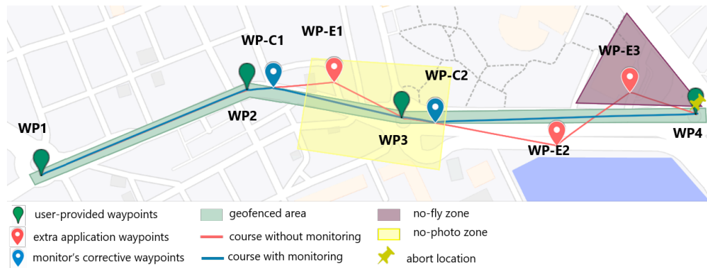
FIGURE 7.8: Simulation experiment with the monitoring mechanism disabled (red line) vs enabled (blue line)
