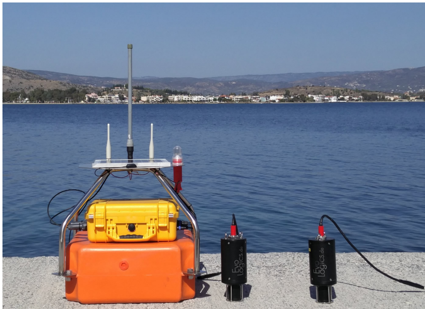
FIGURE A.18: Developed Buoy Alongside a pair of Acoustic Modems by Evologics
