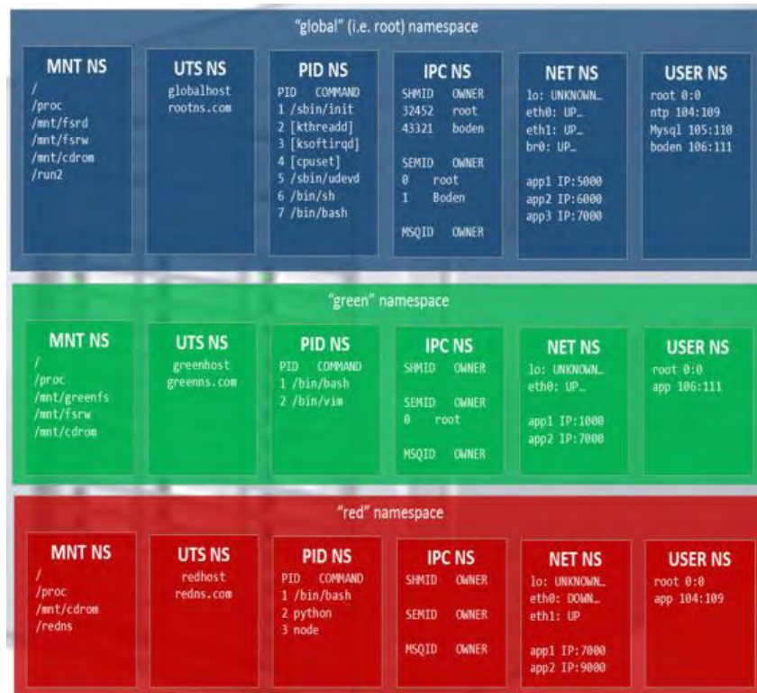
Figure 5 : Linux namespaces conceptual view
