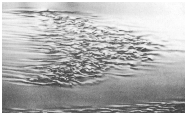
Figure 2.4: Photograph of turbulent spot in a transitional boundary layer, flow from left to right [9].
