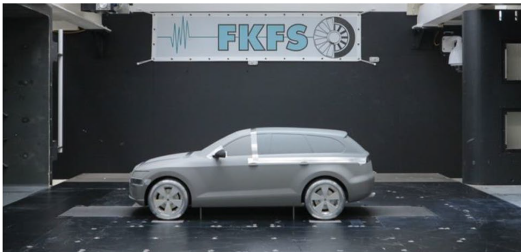
Figure 5.4: The AeroSUV model inside the FKFS windtunnel and the 5-belt system [1] ( edited by the author ).
