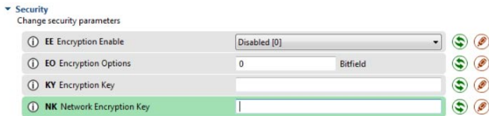
Figure 3.9: X-CTU XBeE security configuration.
