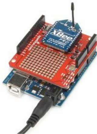
Figure 3.7: the XBee shield, to connect the XBee with UNO
