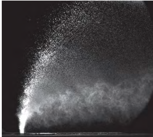
Figure 1.16: Phenomenon of spatial bifurcation of the spray in cross flow (for low GLR)(Sinha, Surya Prakash, Madan Mohan, & Ravikrishna, 2015)
