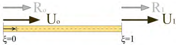
Fig. 66 Fixed-Fixed bar. Subjected to axial displacements u(\xi = 0) = U_0 \hat{x} and u(\xi = 1) = U_1 \hat{x} while the double forces at its ends are prescribed
