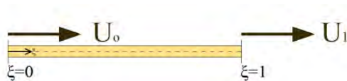
Fig. 68 Fixed-Fixed bar subjected to displacements u(\xi = 0) = U_0 \hat{x} and u(\xi = 1) = U_1 \hat{x}
