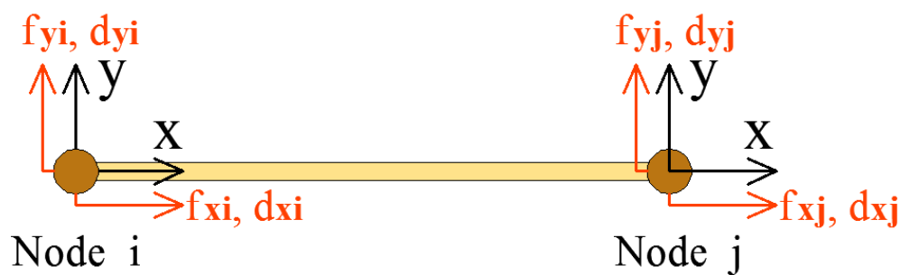
Fig. 128 Forces and displacement vectors expressed in the local coordinate system of a classical bar
