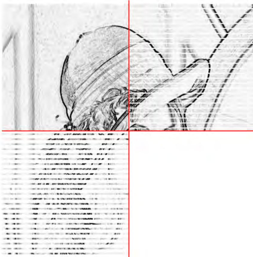
FIGURE 3.4: Different levels of perforation for the Sobel benchmark. Accurate execution, Perforation of 20%, 70% and 100% of loop iterations on the upper left, upper right, lower left and lower right quadrants respectively.
