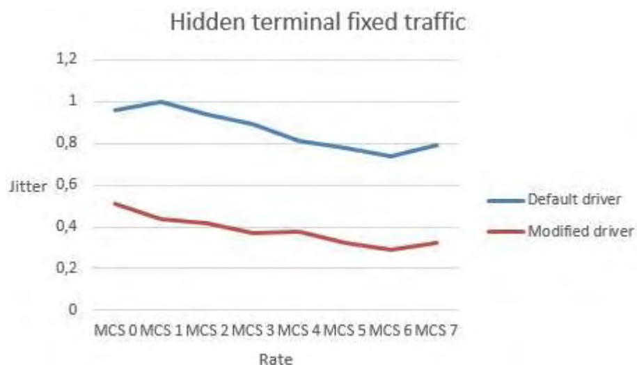
Figure 3-47: Jitter improvement of modified driver in hidden terminal scenario where the traffic of the hidden link is constant to 5 Mbps
