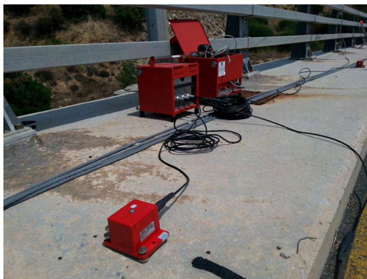
Figure 4.10: Uniaxial accelerometer, junction box, and unit including recorder, battery pack and GPS module
