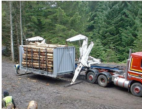
Figure 24. Sidelifter, from http://www.konecranes.com/equipment/lift-trucks/reach-stackers
