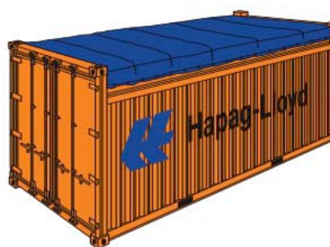
Figure 32. 20 feet open top container, from https://www.hapag-lloyd.com/en/products/fleet/container.html .
