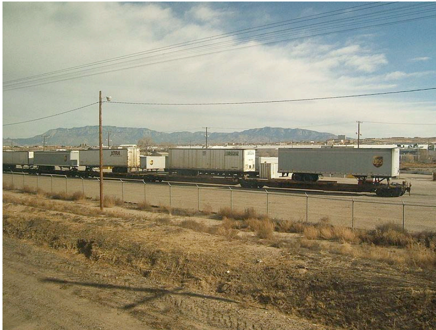
Figure 44. Highway semi-trailers in piggyback service at Albuquerque, New Mexico, from https://en.wikipedia.org/wiki/Intermodal_freight_transport#/media/File:Roadrailleurs.jpg .
