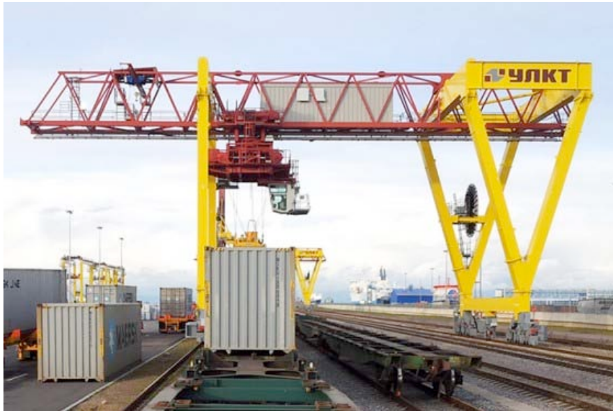
Figure 18. Rail Mounted Gantry Crane (RMG), from https://www.liebherr.com/en/rou/products/maritime-cranes/port-equipment/rail-mounted-stacking-cranes/rail-mounted-gantry-cranes.html .
