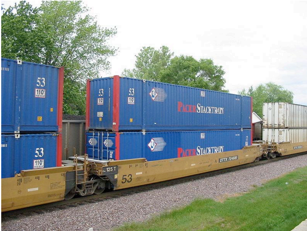
Figure 43. Double-stacked container well cars, from https://en.wikipedia.org/wiki/Well_car#/media/File:DTTX_724681_20050529_IL_Rochelle.jpg
