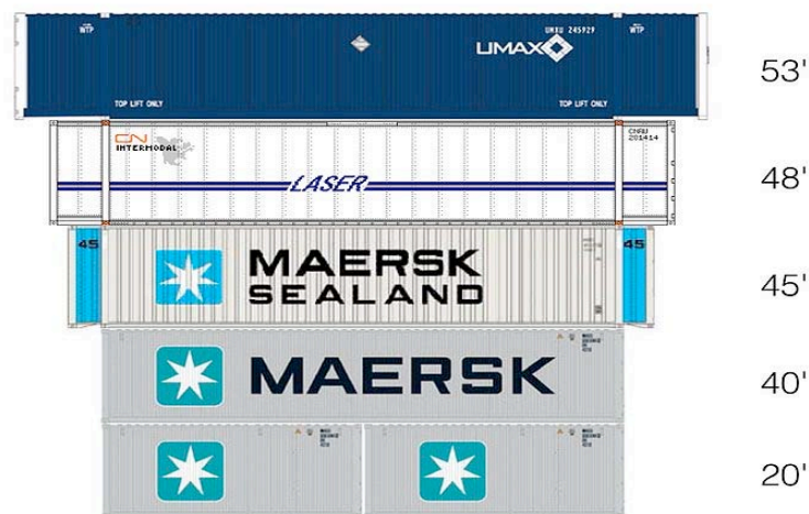
Figure 28. Commonly used container lengths, from https://commons.wikimedia.org/w/index.php?curid=41113427 .
