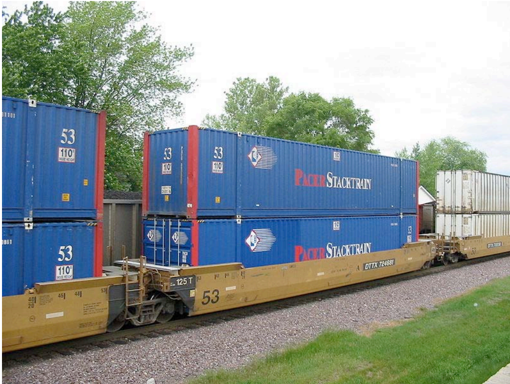
Figure 43. Double-stacked container well cars, from https://en.wikipedia.org/wiki/Well_car#/media/File:DTTX_724681_20050529_IL_Rochelle.jpg
