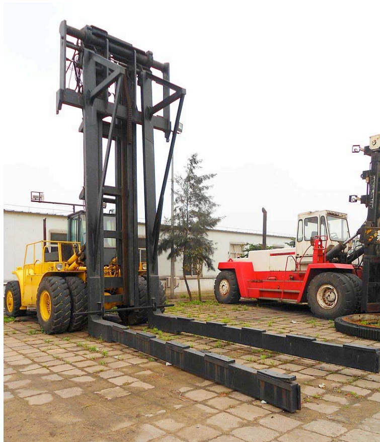
Figure 25. A straight mast container handler at Haikou Xiuying Port, Hainan, China, from https://en.wikipedia.org/wiki/Forklift#/media/File:Straight_mast_container_handler_02.jpg .
