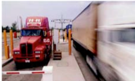
Figure 26. Automated Gate System: driver clearance post,
