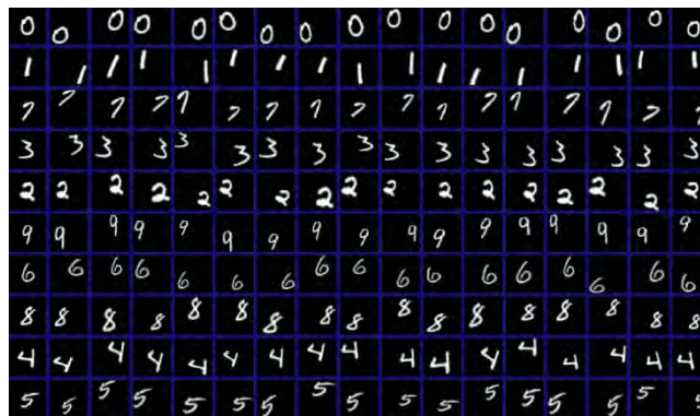
Figure 20 Grid of 10x17 artificially transformed 40x40 digits of the first column and their 16 variations from affNIST dataset [35].
