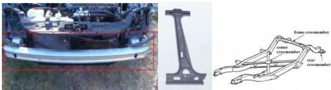
Figure 1.1: The applications of TRIP steels in automotive industry, in the [left] picture front bumper, [center] picture B pillar, [right] cross members.
