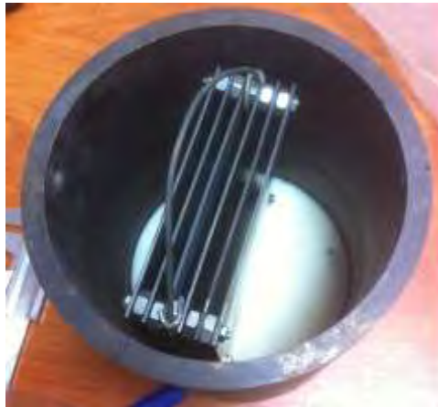
Figure 3.7: Placement of steel samples inside the tank prior to the heat treatment process
