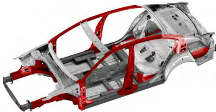
Figure 2.2: Car components manufactured from Trip steels [2]
