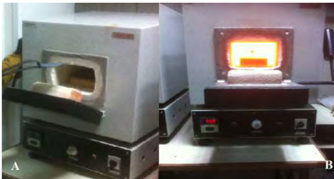
Figure 3.7: Front load furnaces A) for preheating, B) for austenitization process
