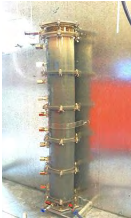
Figure 5.22 Experimental set up for the 1m column injection test (Test No8), where the whole 1m column may be observed.
