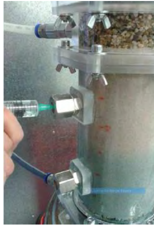
Figure 5.10 Pore fluid sampling when the CS front is located at a height of 10cm at the time of the sampling and it is before (upstream of) the sampling port.
