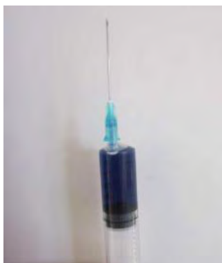
Figure 5.7 Syringe used to extract small samples of the dyed pore fluid during 1D column injection tests.
