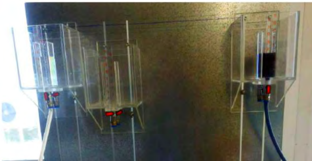
Figure 5.12 Set up of vertical 1D injection tests for the main set of tests using small inlet and outlet chambers.
