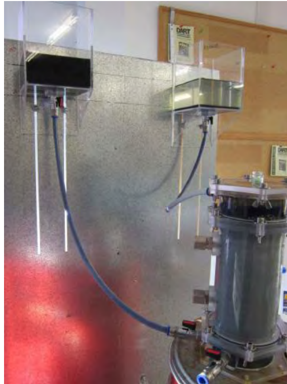
Figure 5.8 Set up of vertical 1D injection tests (large chambers). Observe that breakthrough has been performed (all the sample is dyed blue) and the heavier and more viscous CS can be clearly seen at the bottom of the outlet chamber, as a thin layer below the water-filled chamber.
