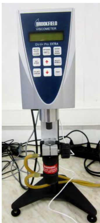
Figure 4.1 Brookfield LVDV-II+PX rotational viscometer at the University of Thessaly.
