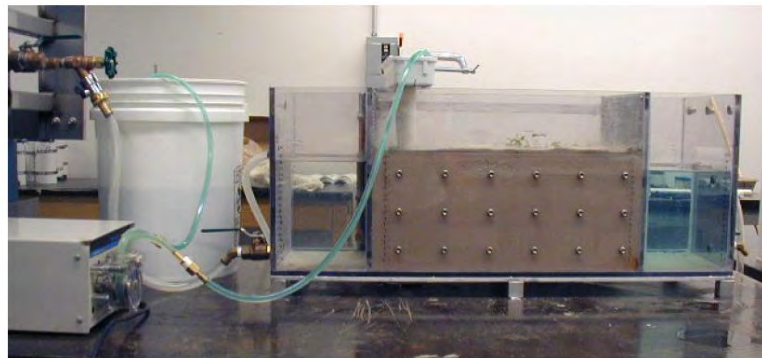
Figure 2.18 Experimental set up for 2-D injection tests (Koch 2002).
