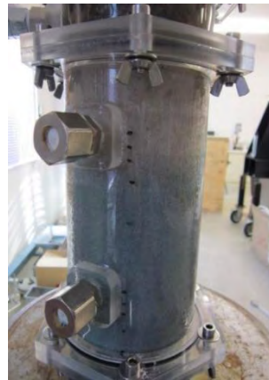
Figure 5.15 Snapshot of CS front at the end of Test No4. Observe that breakthrough was not attained in this test and this clearly depicted by the change of color within the sand sample.
