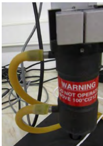
Figure 4.5 Connection of water bath to viscometer.
