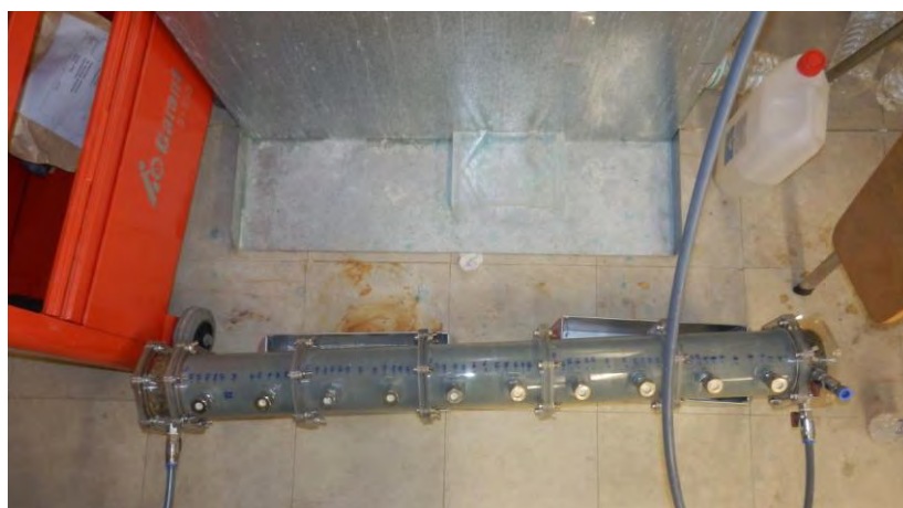
Figure 5.54 View of CS front location at the end of the horizontal injection test.
