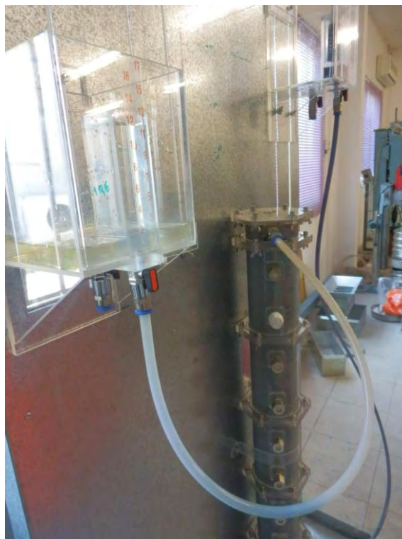
Figure 5.25 Full coverage (breakthrough) of 1m sand column with injected dyed blue CS solution in Test No8.
