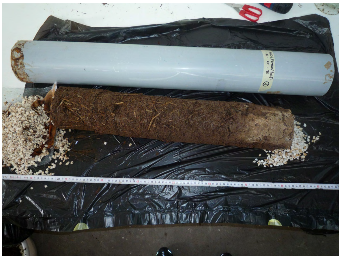
Photograph 3.2: The packing material of the leaching columns after completion of the treatment period.
