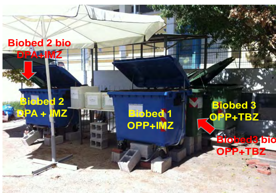
Photograph 4.4. The 5 pilot biobeds and the treatment employed in each of them.
