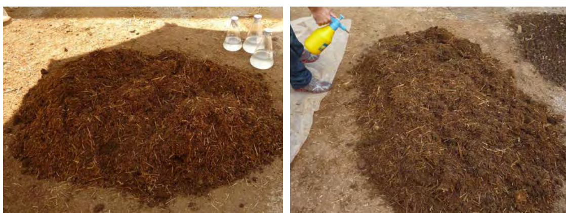
Photograph 4.3. The application of tailored-made bacterial inocula in the biobed packing material of pilot biobeds "biobed 2bioaug" and "biobed 3bioaug".
