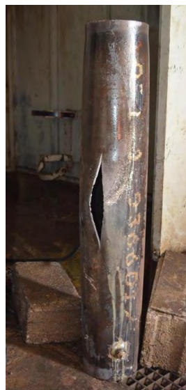
Figure 3-63: Rupture of perfect \text{Ø} 168.3/4.78 specimen
