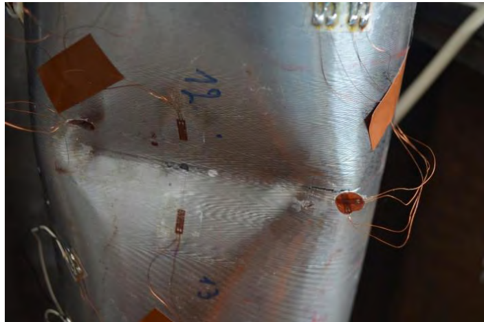
Figure 3-45: Pipe wall rupture of specimen SP9d-4pb due to cyclic bending loading at the dent “ridge”.
