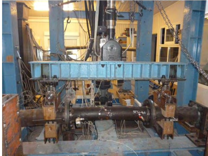
Figure 3-19: Four-point bending experimental set-up.
