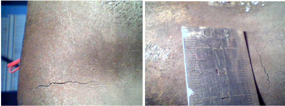
Figure 3-44: Final cracks detected at the buckle “ridges” on (a) SP1d at 1400 Cycle and (b) SP3d at 1090 Cycle (3cm-long crack)
