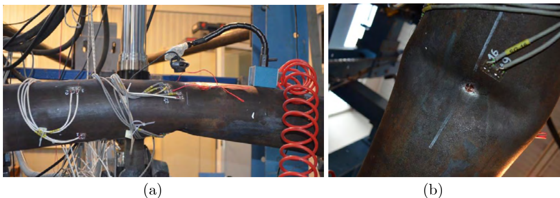
Figure 3-43: (a) Side view of dented specimen SP1d and (b) detail of the buckle development at the opposite of the dent during monotonic and cyclic 4-point bending
