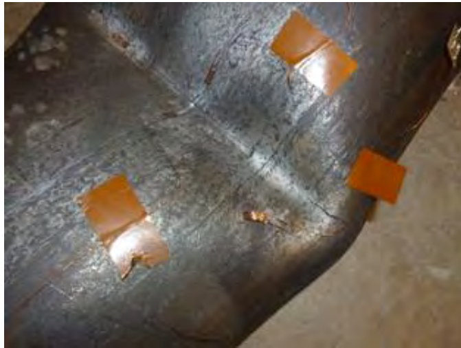
Figure 3-38: Pipe wall rupture of specimen SP5d due to cyclic bending loading at the dent "ridge".
