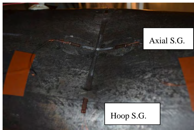
Figure 3-30: Denting region of SP5d specimen after load removal
