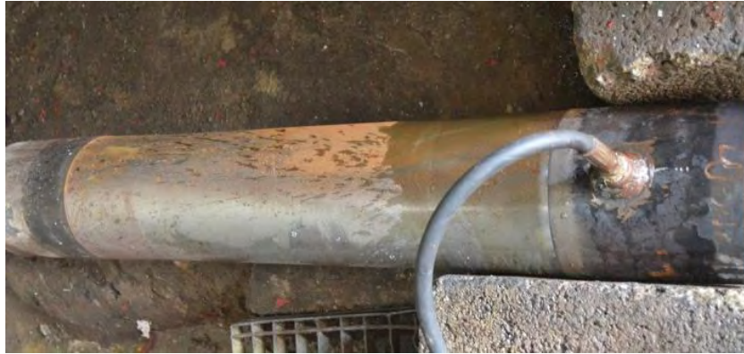
Figure 3-26: Pressure application on specimens \text{Ø}165/3 .
