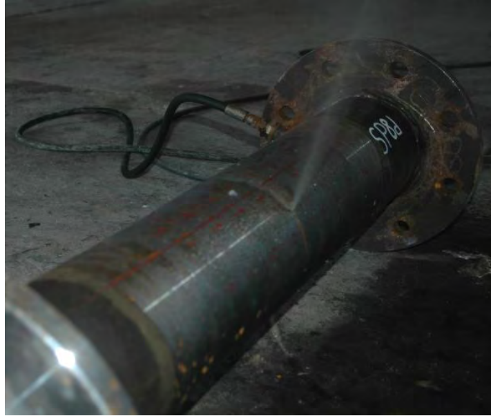
Figure 3-57: Rupture \text{Ø}165/3 pipe specimen SP8d due to cyclic internal pressure; wall rupture location at the "ridge" of the dent location.
