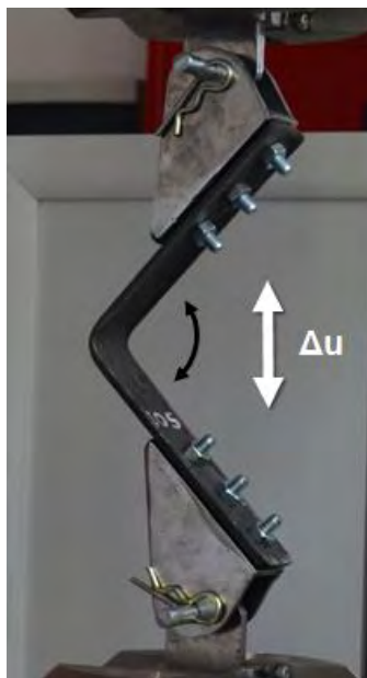
Figure 5-3: Loading and test configuration of strip specimens
