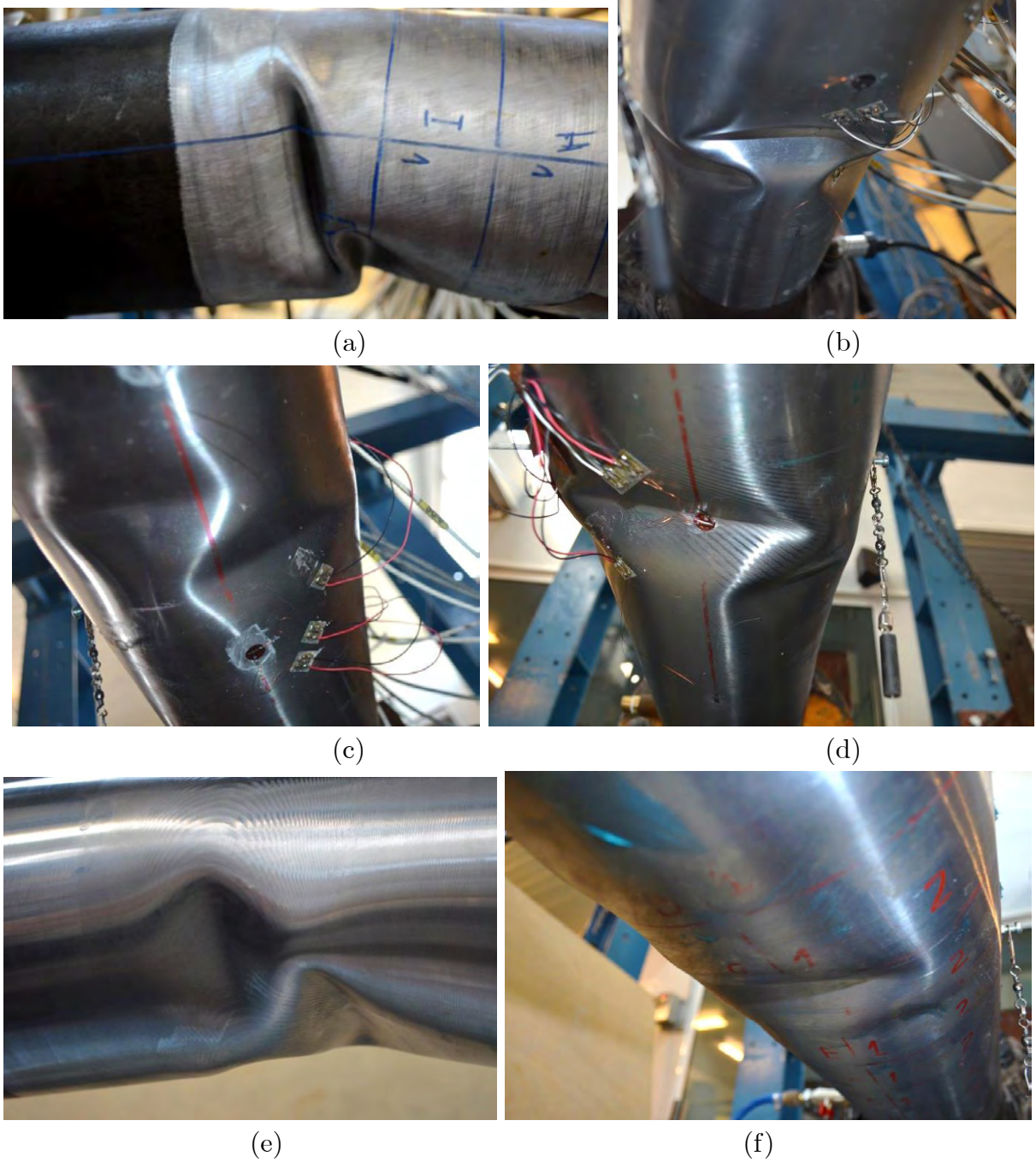
Figure 3-52: Detail of the non-symmetric buckle for (a) SP3b, (b) SP4b and (c) SP5b (d) SP6b (e) SP7b and (f) SP8b specimens.
