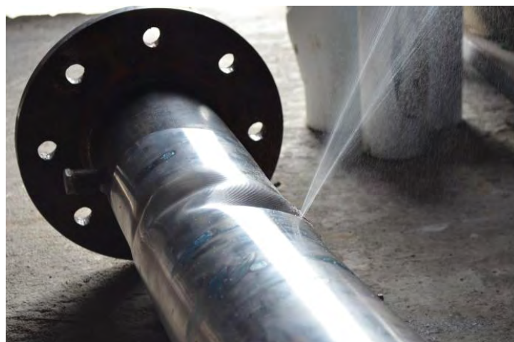
Figure 3-59: Ruptured \varnothing 165/3 pipe specimen (SP7b) due to cyclic internal pressure; wall rupture location at the buckle location
