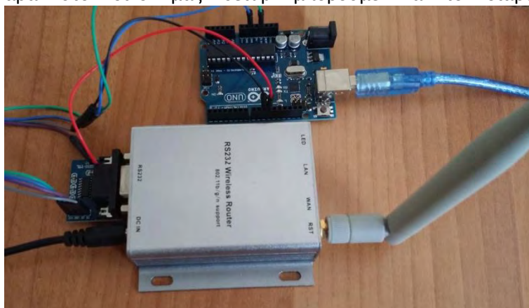
Rs232 Wifi Server (Serial to Ethernet/wifi converter)
