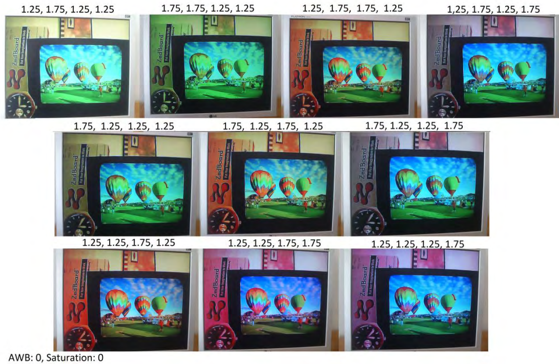
Figure 2.15: Different Options for Fix Gain Control (Red, Green, Blue)
