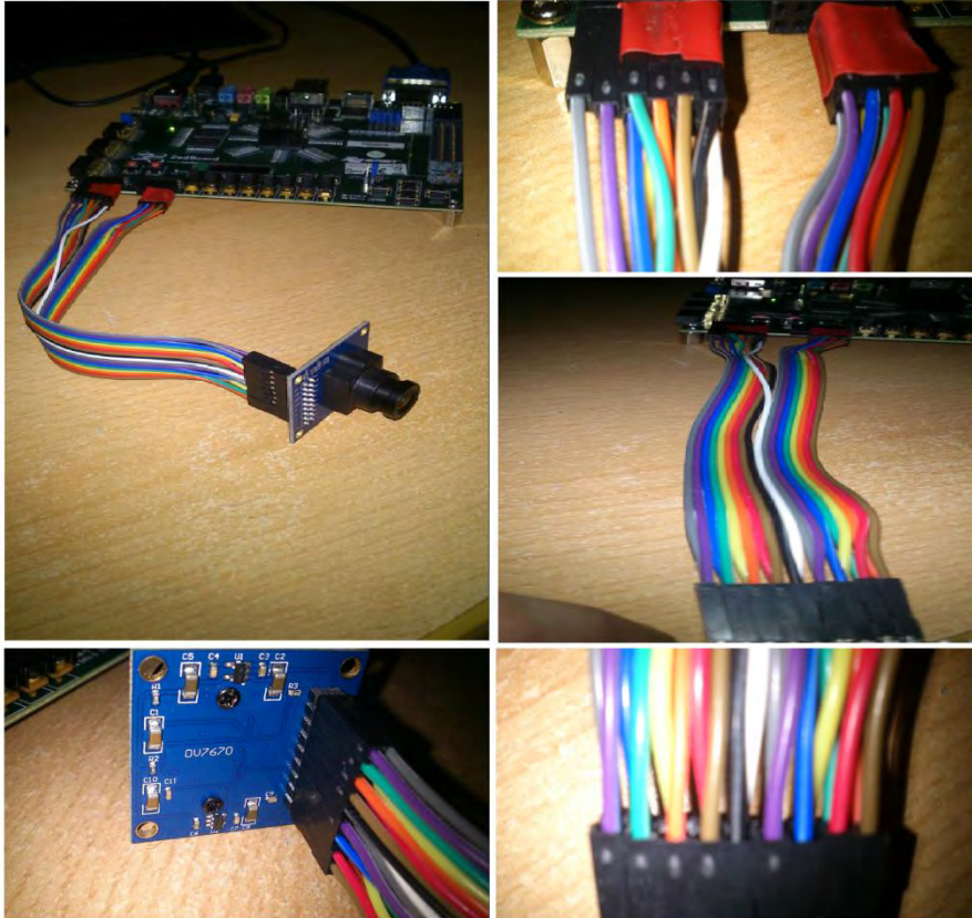
Figure 3.3: ZedBoard and Camera Interconnection
