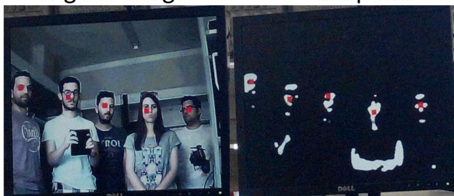
Figure 4.4: Face Detection and Tracking for 3-5 Faces
