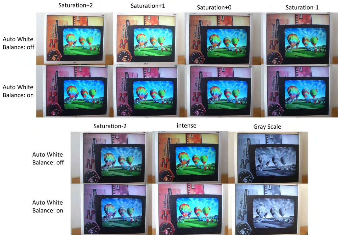
Figure 2.10: Different Options for Saturation and Auto White Balance (AWB)
