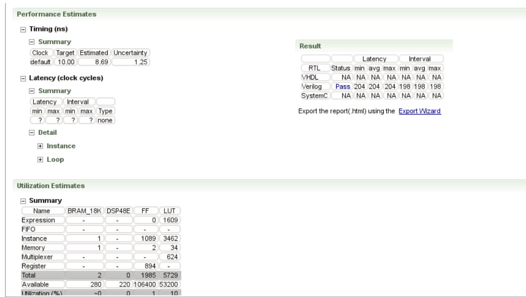
Image 6.5 High Level Synthesis with loop unroll factor of 2
