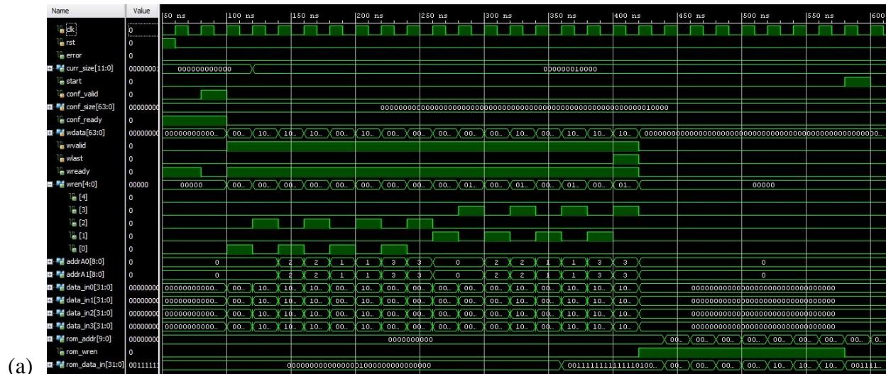
Figure 3.26 (a) and (b) shows waveforms of axi unit operations for 16-point FFT.
