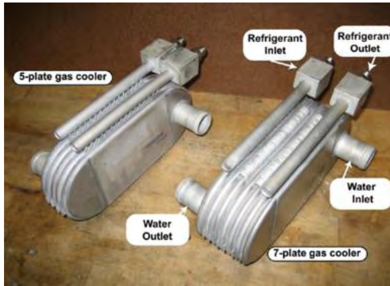
Figure 4. A photo of a heat exchanger that is used as gas cooler
