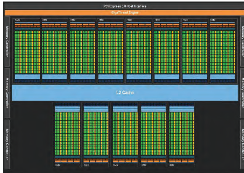
Figure 2-1: Architecture of the NVIDIA Tesla K20 GPU.
