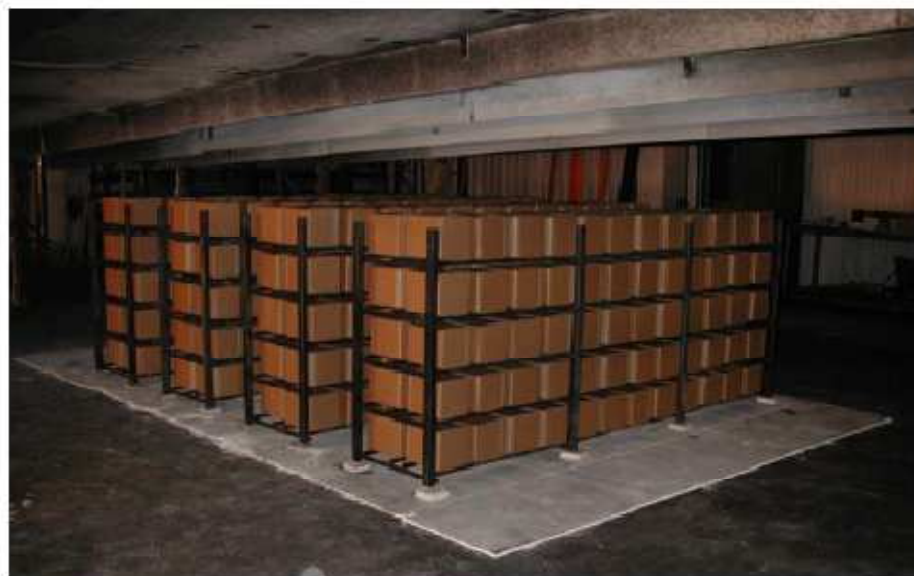
Fig. 8.7 Experimental setup of the rack units (Lönnermak and Ingason,2005)
