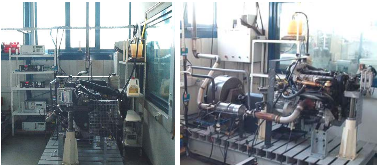
Figure 7.1 Large scale engine test bed
