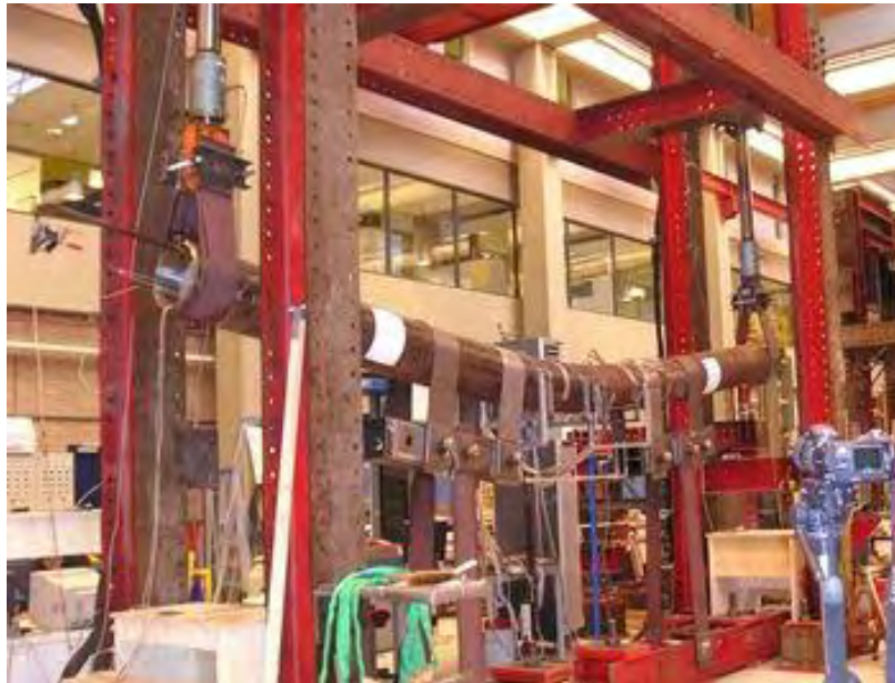
Figure 74: Four-point bending test of lined pipes [13].
