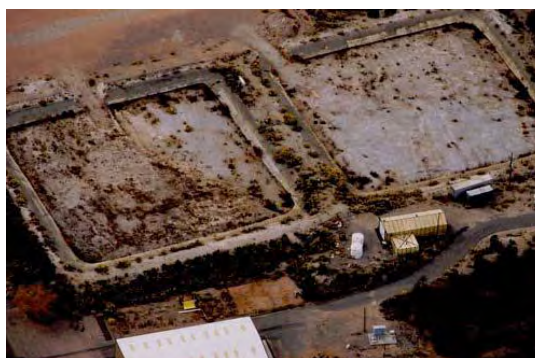
Figure 1.17. Evaporation ponds used for the disposal of pesticide-contaminated wastewaters (source: LANL, “Aerial tour of Los Alamos National Laboratory,” Los Alamos Study Group, Albuquerque, 2004. http://www.lasg.org ).
