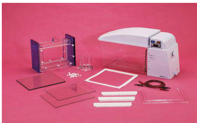
Figure 2.3. The DGGE system used (source: INGENYphorU-2, Instruction manual).
