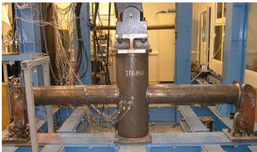
Figure 5.2: Test configuration for IPB loading.
