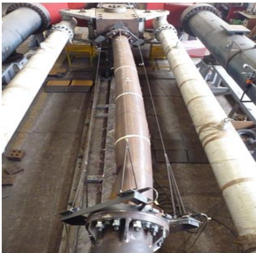
Figure 3. 1: Experimental set-up for tube bending [Bursi (2012)].
