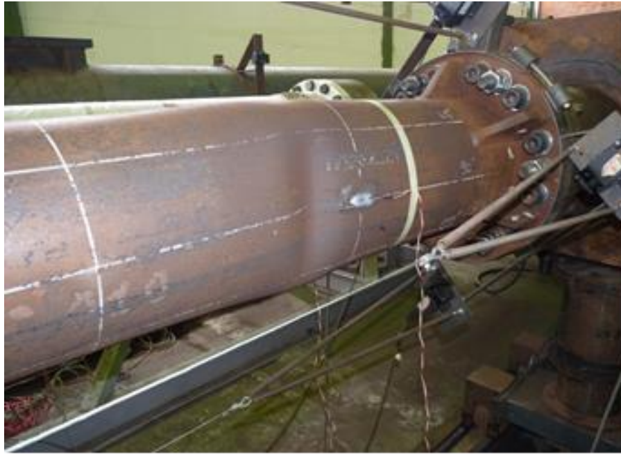
Figure 3. 4: Local buckling modes: (a) Specimen No. 1, (b) Specimen No. 2 [Bursi (2012)].
