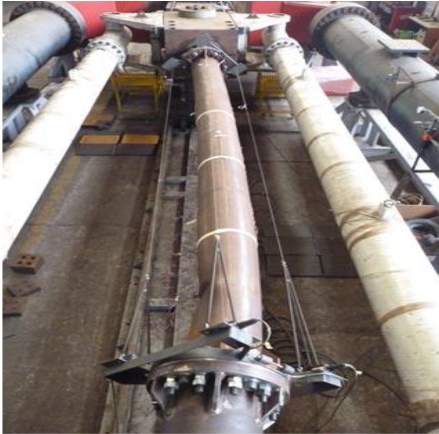
Figure 3. 1: Experimental set-up for tube bending [Bursi (2012)].
