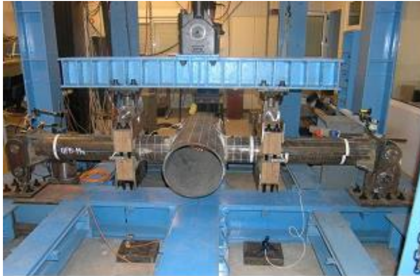
Figure 5.3: Test configuration for OPB loading.
