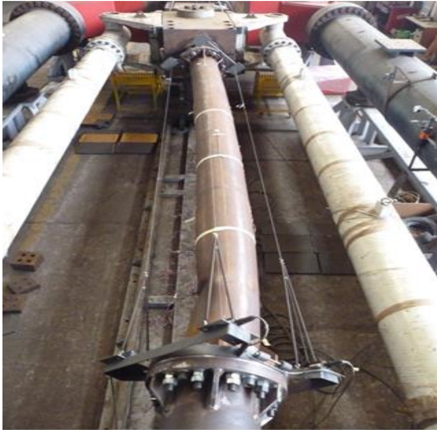
Figure 3. 1: Experimental set-up for tube bending [Bursi (2012)].
