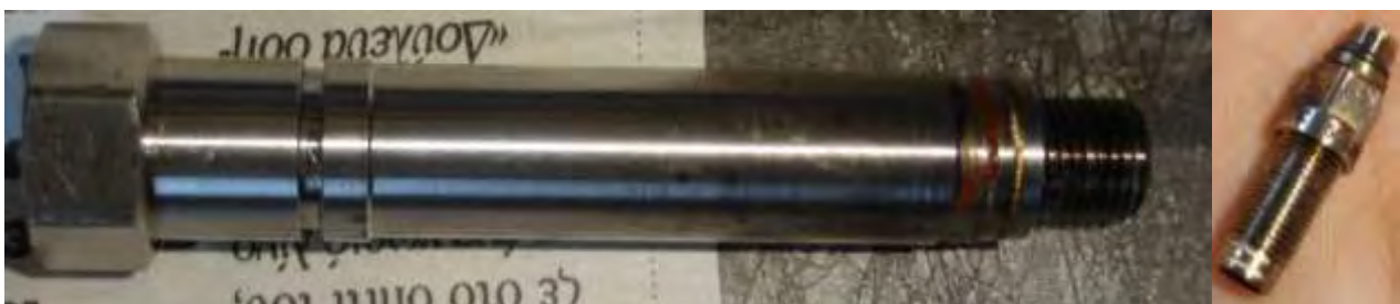
Figure 6.10. Mounting sleeve 6525Asp (left) and piezoelectric sensor 6052B1 (right).
