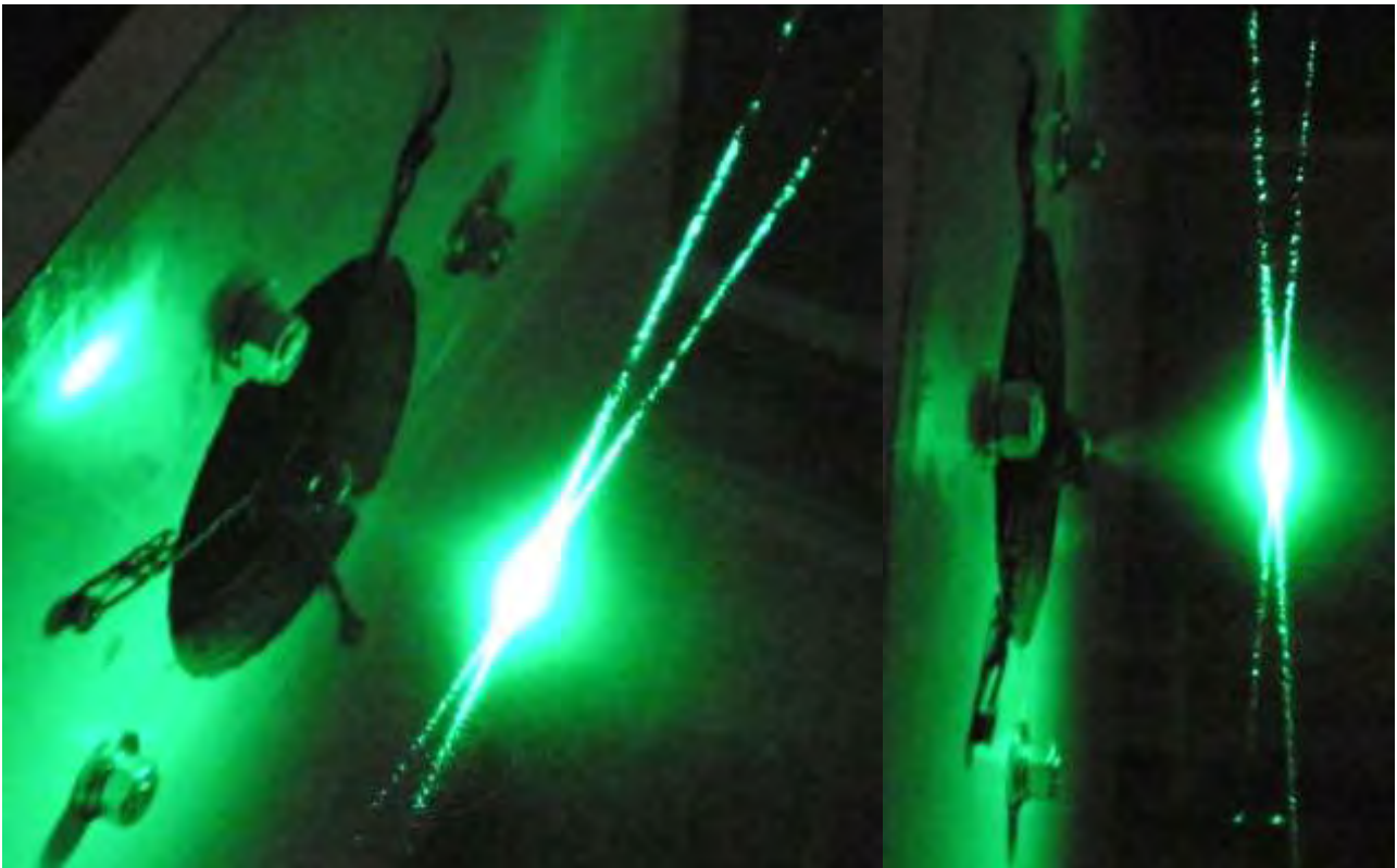
Figure 9.3. Low pressure diesel spray. Green laser beams and cross-section area (measurement volume) are clearly observable.
