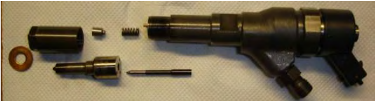
Figure 8.11. Common rail injector components. From right to left we have, injector body including supply and return fuel line, spring, plunger, nozzle body including needle, nozzle house and washer.
