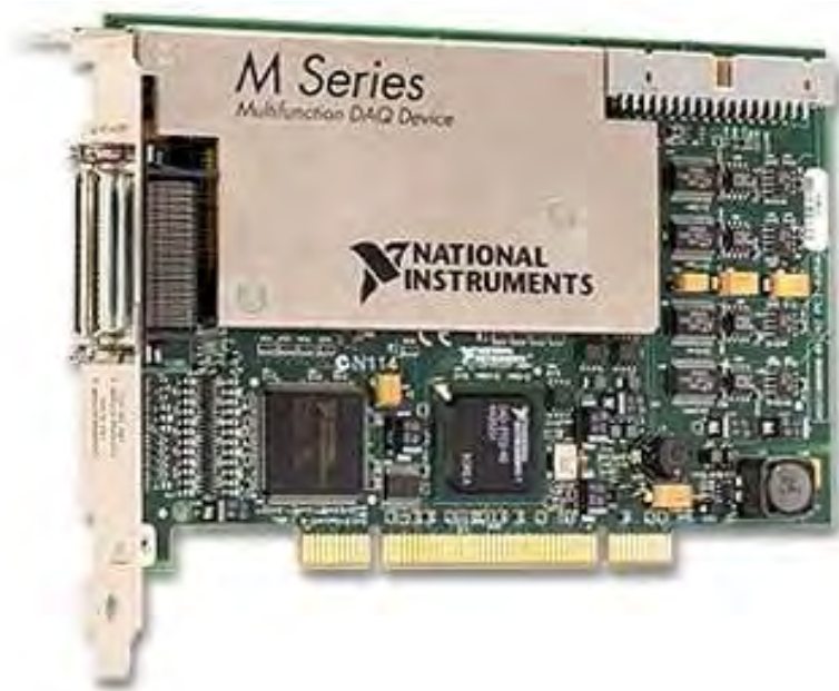
Figure 6.11. PCI-6259 high speed data acquisition card.
