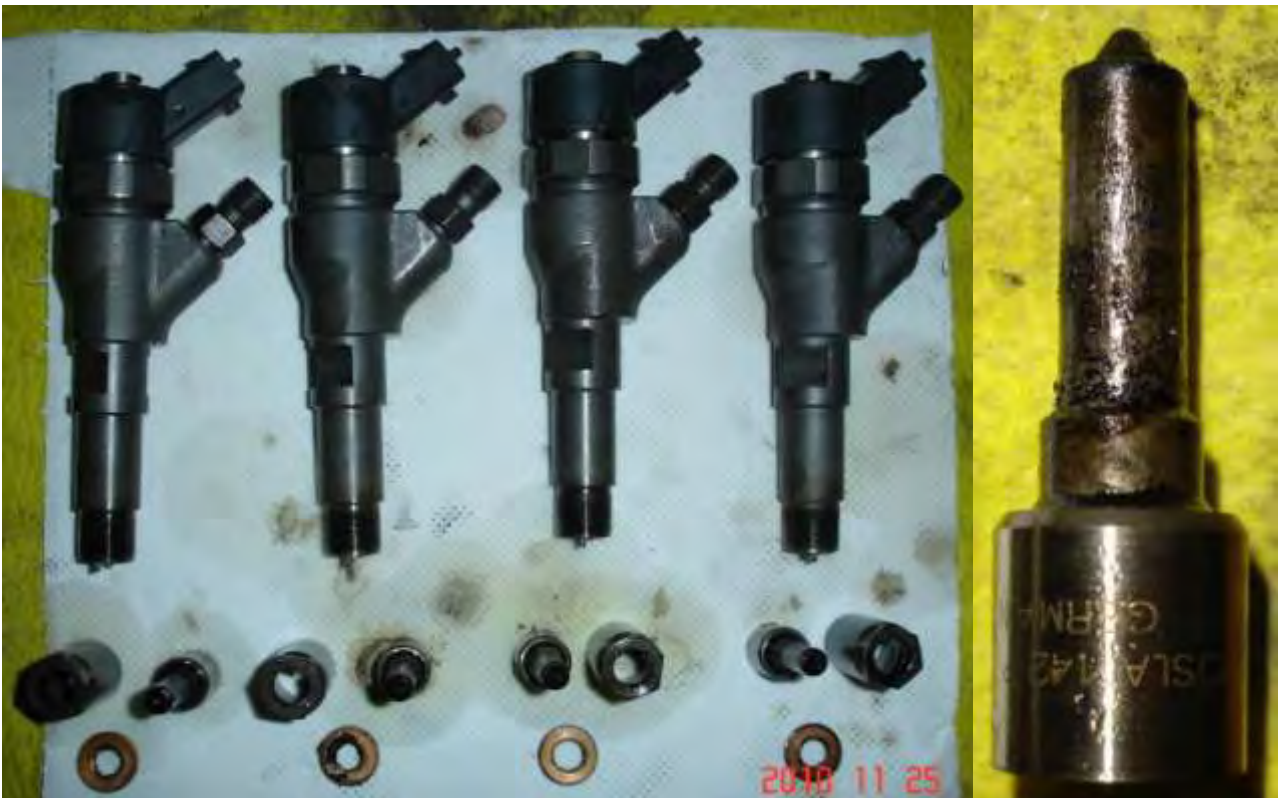
Figure 8.9. Disassembly view of the injectors (left) and closer view of the nozzle (right).
