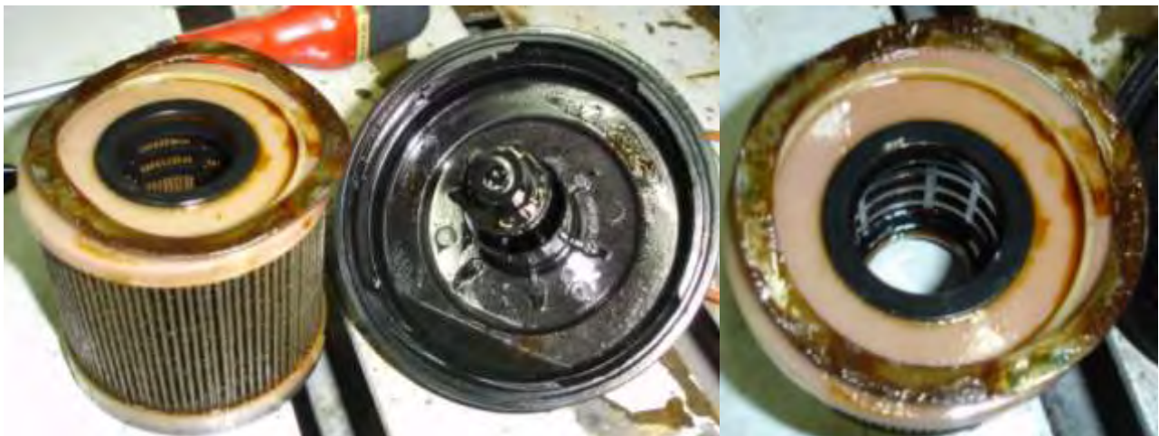
Figure 8.2. Fuel filter condition after 30 h operation with B70 fuel.
