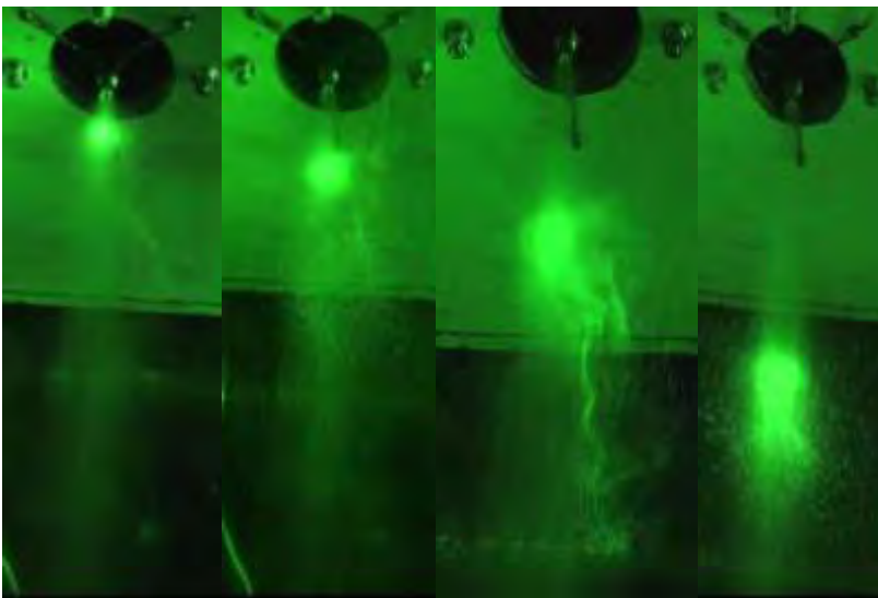
Figure 9.26. Spray evolution injections using low pressure nozzle for B100 fuel at several positions from the tip of the nozzle and under specific injection conditions. P_{inj} = 10 bar, P_{amb} = 1.01 .
