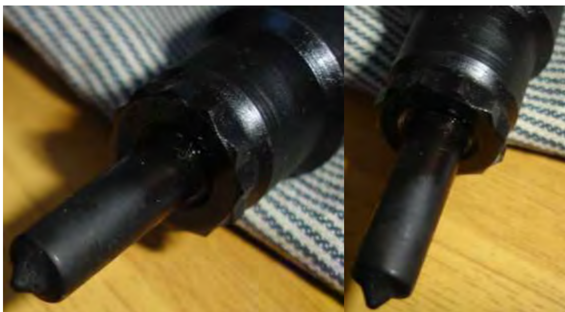
Figure 8.19. RF91 injector closer view after 40 h operation with conventional diesel fuel (B0 and 0 ppm fuel additive).
