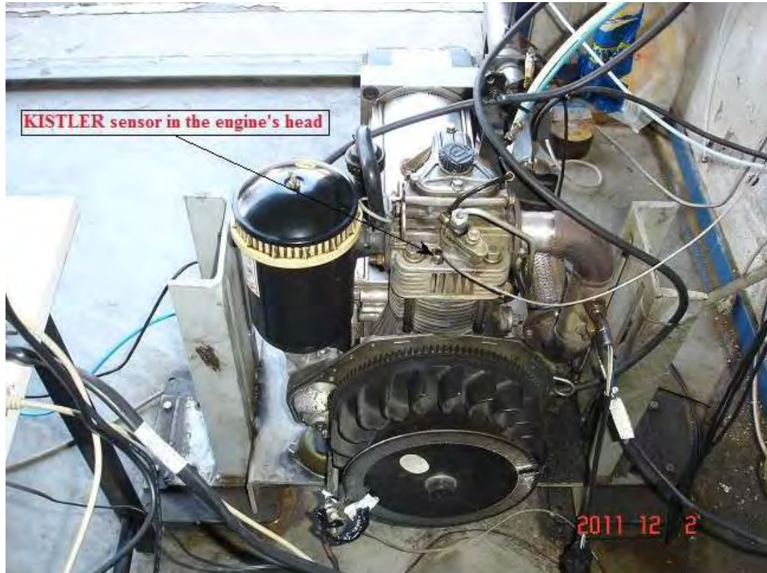
Figure 3.12: KISTLER piezoelectric sensor in the engine's cylinder head.
