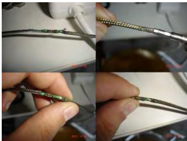
Figure 3.26: KISTLER's cut off wire due to a short circuit.
