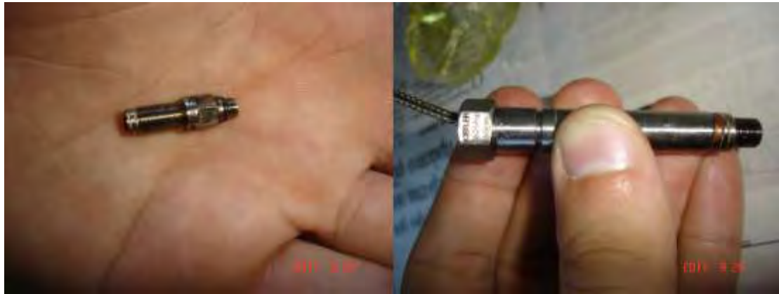
Figure 3.13: KISTLER 6052B1 (left) mounted over a KISTLER 6525ASP20-50 head (right).
