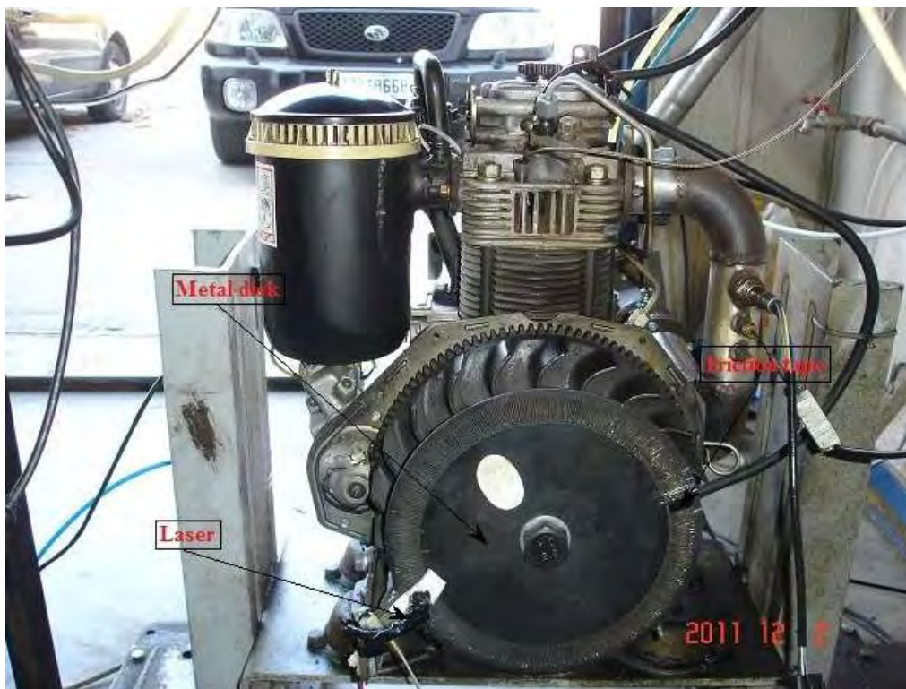
Figure 3.17: Metal disk adapted to the engine's crank and laser.
