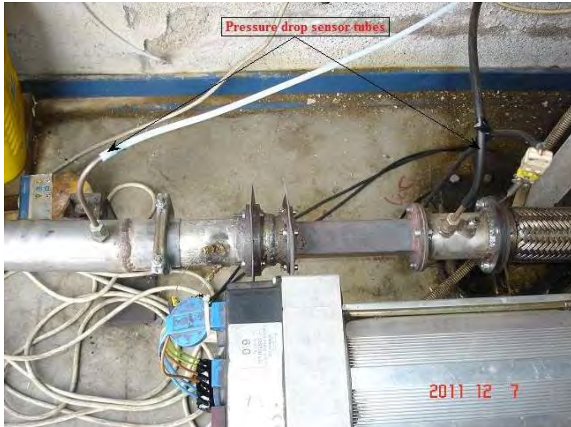
Figure 3.15: Pressure drop sensor tubes adapted to the exhaust.
