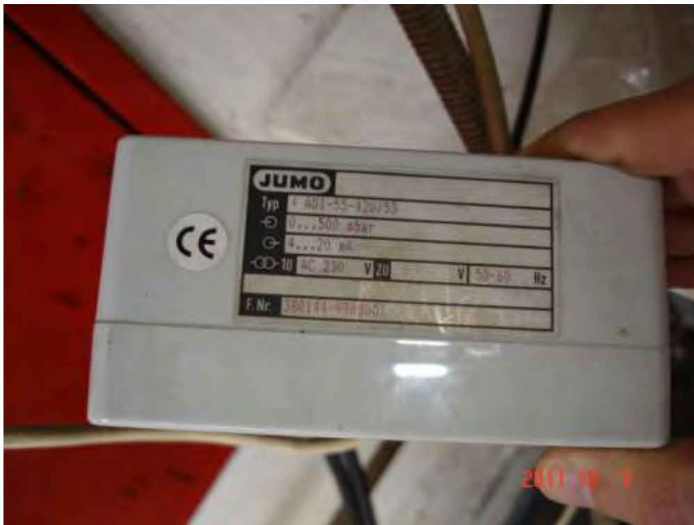
Figure 3.16: Pressure drop sensor.
