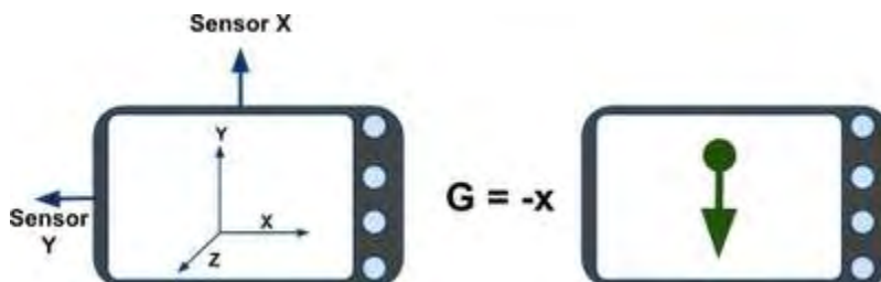
Figure 18: The sensor coordinate system never changes, so in G = -x means that gravity is aligned with the device's negative-X axis.
