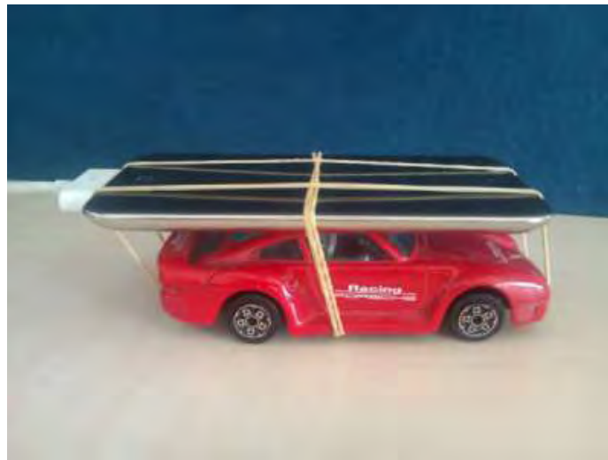
Figure 37: Mounted iPod on toy car, for tracking acceleration and velocity on Y axis
