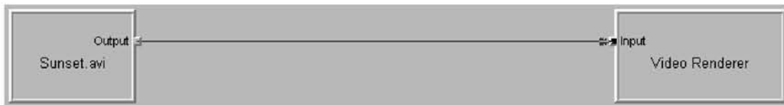
Figure 2-12. A source filter can't be connected directly to a renderer filter, unless...
