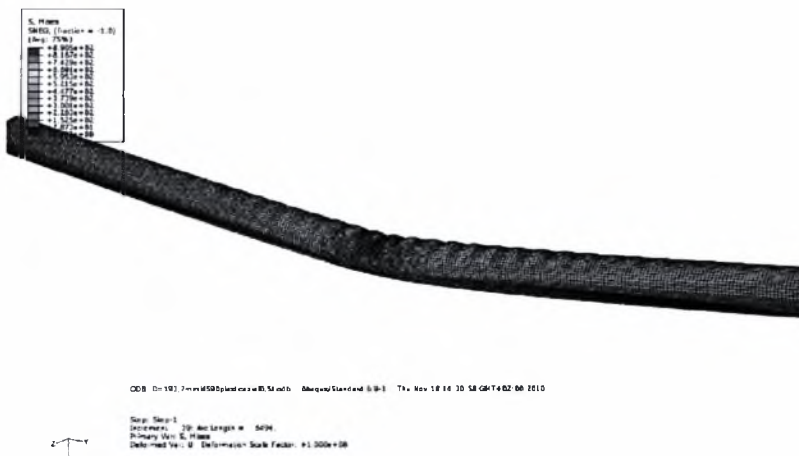
Figure C.2.2 Failure mode for the wrinkled tube with w_0/t=0.5
