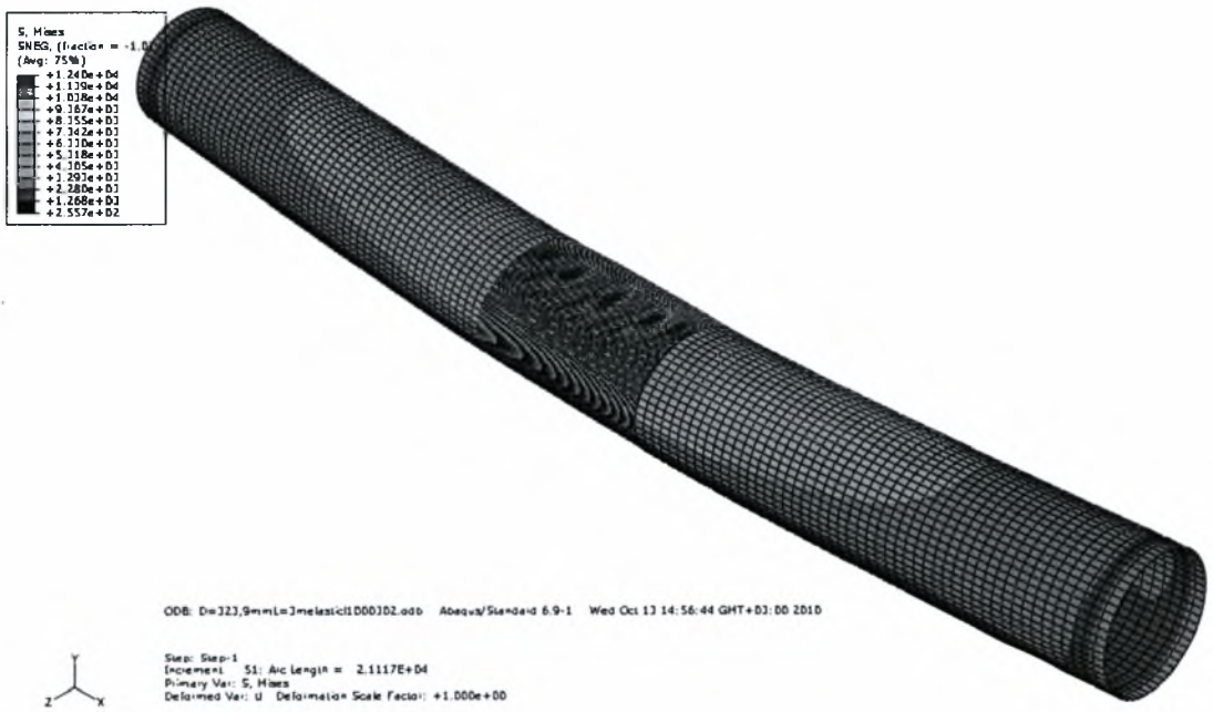
Figure A.2.3 Post buckling behavior where local buckling occurs wrinkling development, point
