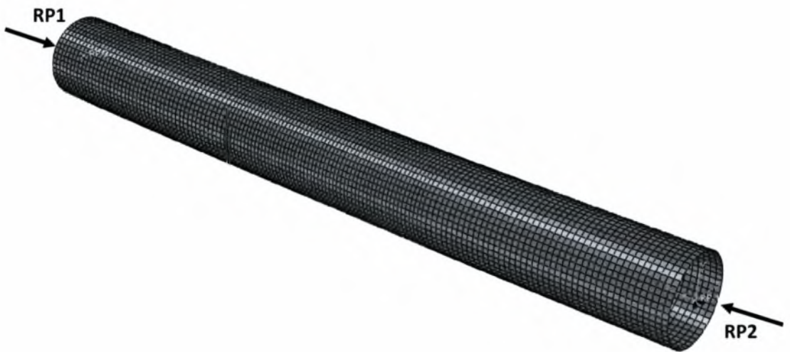
Figure 4.1.2 The finite element model loading under axial compression and boundary conditions
