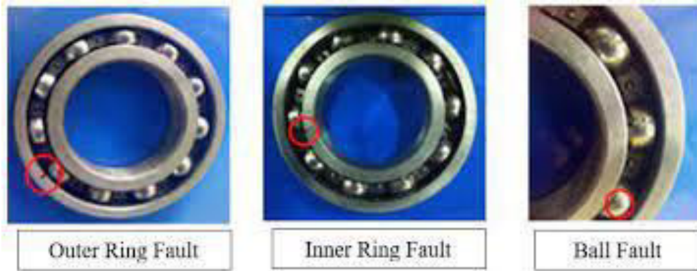
Image 13. [26] Bearings with local the three local faults described in this work.
