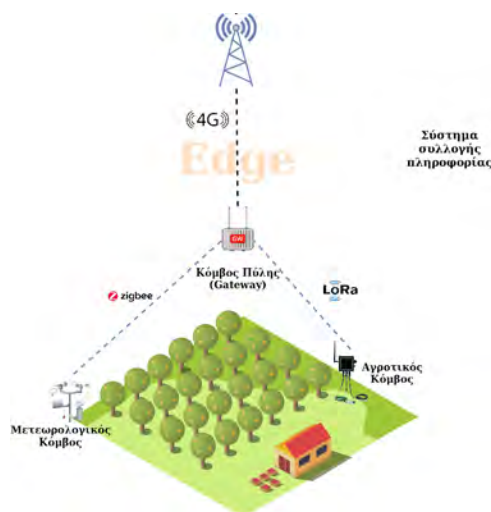
Figure 3.2. The Figure shows the edge devices and how the can communicate with the cloud.
