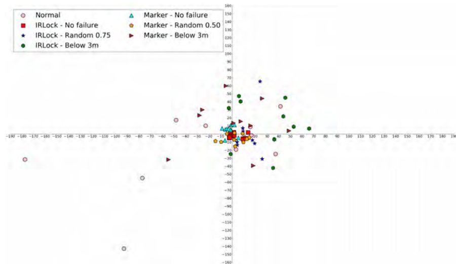
(b) Landing positions relative to the center of the landing target (units in cm).
