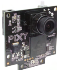
(a) Pixy vision sensor with IRLock filter and specialized firmware.
