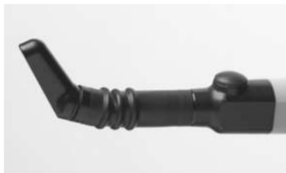
Figure 15: "Hockey stick" linear array ultrasound transducer, the most commonly used during intraoperative ultrasound after CEA.
