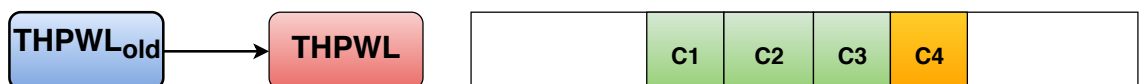
(d) Step 4: Restore the old THPWL before continuing with cell's next tentative move
