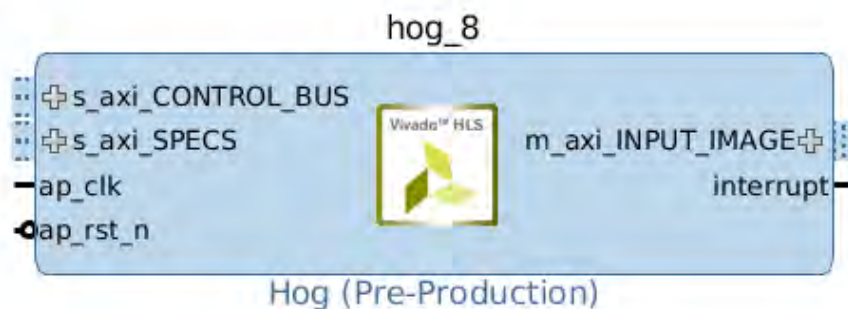
Figure 5.16: Overview of the accelerator's IP ports
