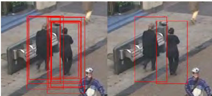
Figure 2.9: Non-maximal suppression reduces the effect of multiple detections of the same pedestrian
