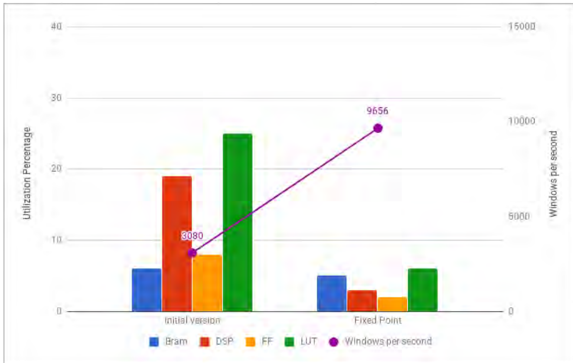
Figure 5.6: Resources vs Latency for the first optimization step
