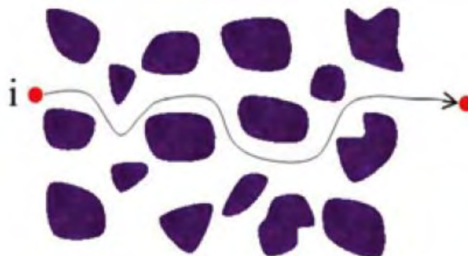
Figure 4.4. Illustration of Knudsen and molecular diffusion in random porous material [16].
