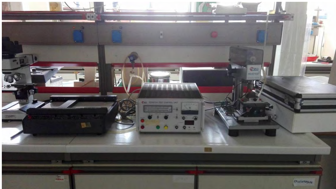
Fig. 10: CSM Revetest Scratch Test Connected with CSM Scratch Test Control Unit equipped with an ABB SE-790 XY plotter
