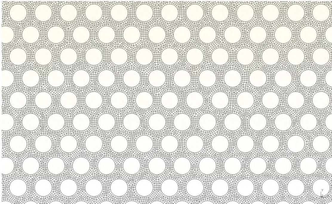
Figure 13: Zoom in internal mesh of unit cell for \varphi_i=0.5 and \varphi_t=0.5
