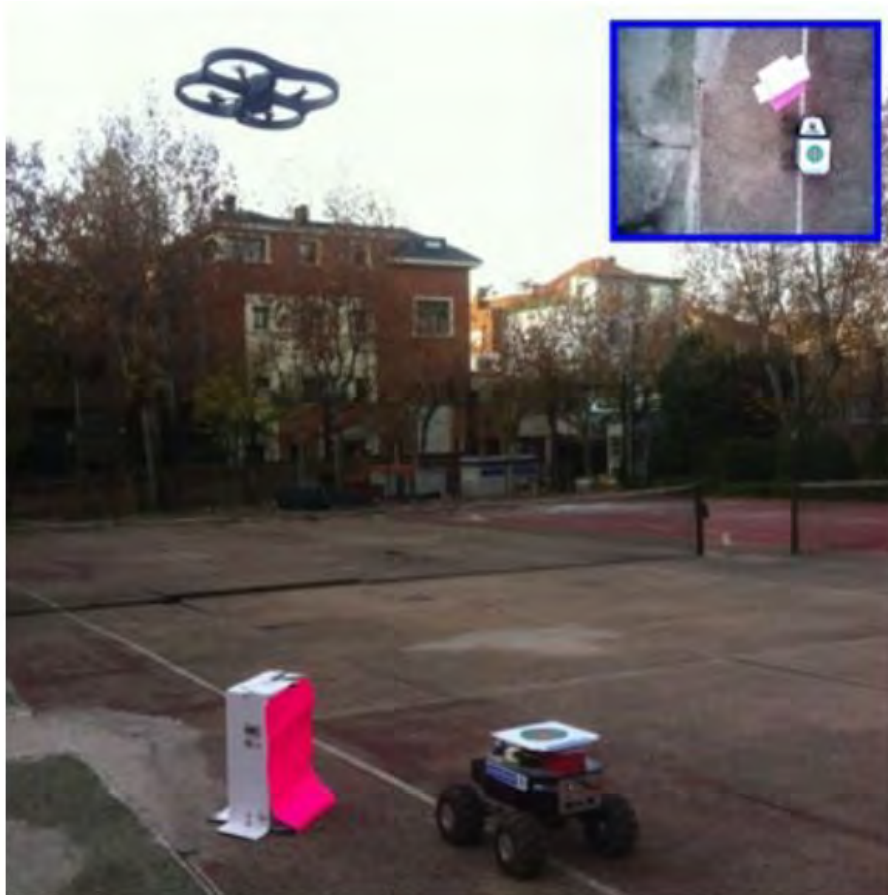
Figure 1.7: A swarm architecture designed for UGVs obstacle avoidance based on aerial observations using UAVs [80].
