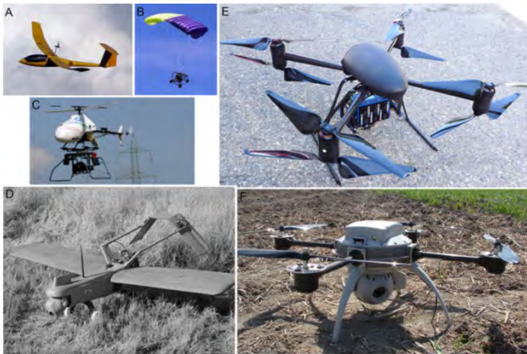
Figure 1.6: A. powered glider, B. powered parachute, C. helicopter, D. fixed wing aircraft, E. Draganflyer X8 quadcopter, F. Aeryon Scout quadcopter [89].
