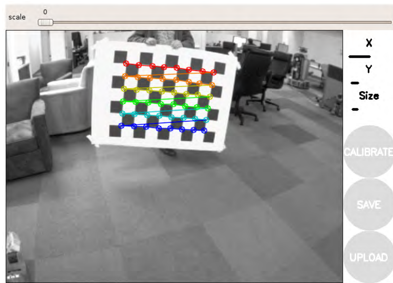
Figure 8.3: The lens calibration chess pattern
