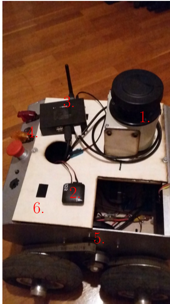
Figure 6.3: Electronics installation on top of the rover
