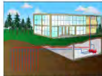
Ground-Coupled WSHP System
