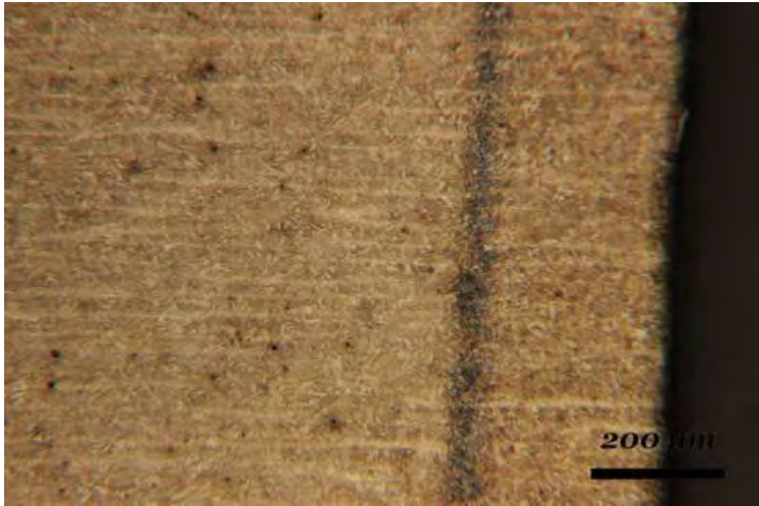
Figure 4.25 (x100) – C3 SPECIMEN'S HAZ, NEAR THE TOP PLATE'S SURFACE
