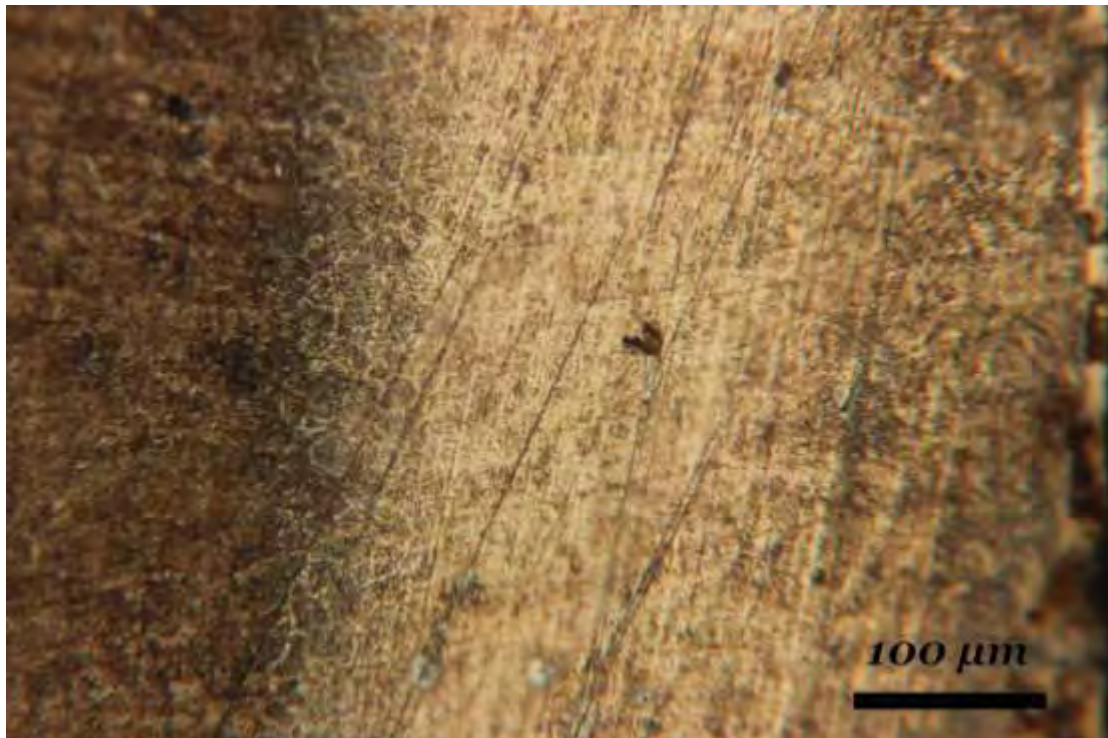
Figure 4.19 (x200) – B4 SPECIMEN'S HAZ, NEAR THE BOTTOM PLATE'S SURFACE
