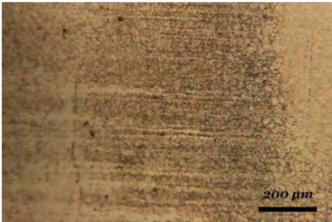
Figure 4.24 (x100) - C2 SPECIMEN'S HAZ, NEAR THE BOTTOM PLATE'S SURFACE
