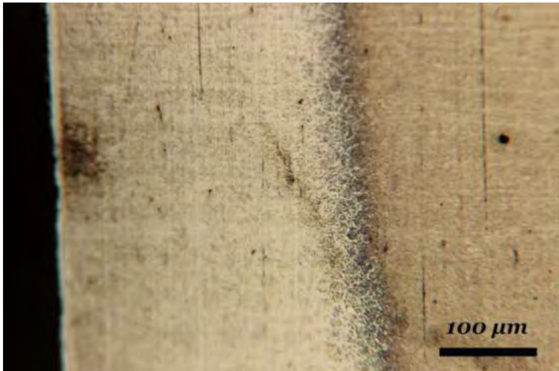
Figure 4.6 (x200) – A2 SPECIMEN'S HAZ, NEAR THE BOTTOM PLATE'S SURFACE
