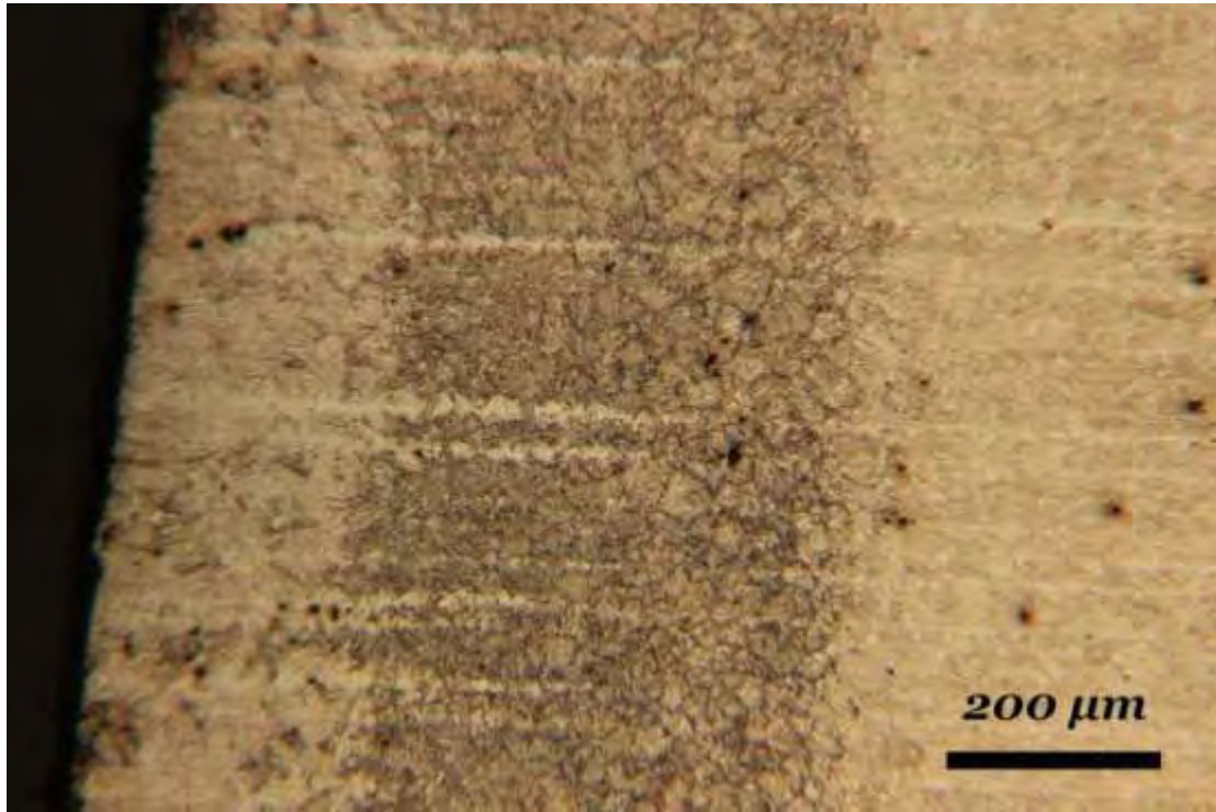
Figure 4.23 (x100) – C2 SPECIMEN'S HAZ, NEAR THE TOP PLATE'S SURFACE
