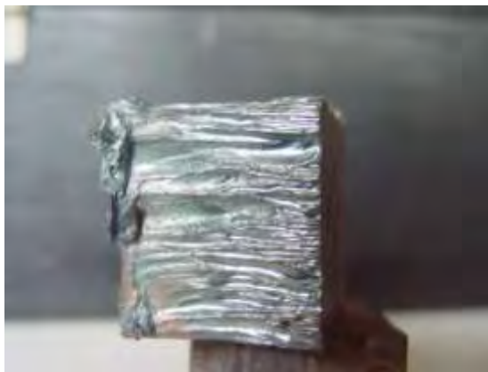
Figure 5.2 – CUT FACE OF SPECIMEN C2
