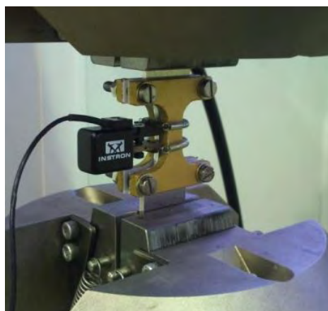
Figure 3.19 Strain controlled fatigue test setup with the use of anti-buckling device.
