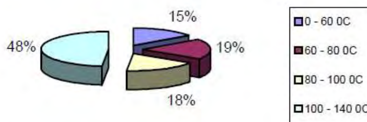
Figure 27: Distribution of thermal energy requirements relative to the process temperature in dairies
