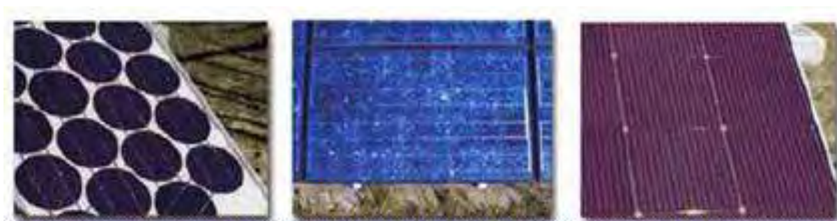
Figure 14: Types of photovoltaic panels (monocrystalline silicon, polycrystalline silicon, amorphous silicon)
