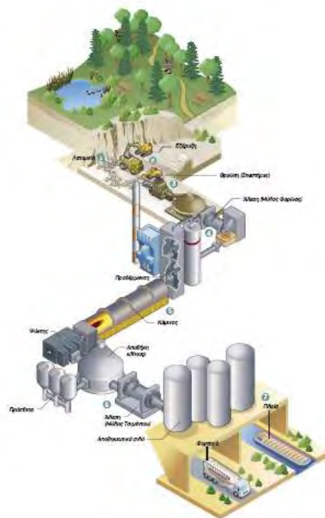
Figure 2.1: Basic flow sheet of cement production
